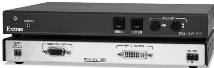
The Extron RGB-DVI 300 is a high performance RGB to DVI scaler that converts incoming analog component video and RGBHV signals to DVI. It accepts HDTV and high resolution computer-video signals, and offers single link DVI output rates up to 1920x1200, including HDTV 1080p/60.
